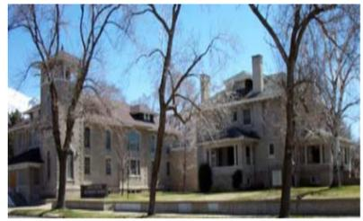
Architect – Unknown, designed in the Prairie/Craftsman style. The front and side porch enclosures have brick rails capped in sandstone with roofs supported on concrete columns and brick piers. The foundation is concrete, which has been scoured to resemble block. The walls are set in a stretcher bond with simulated quoins at the corners, achieved with grouped extruding brick.
